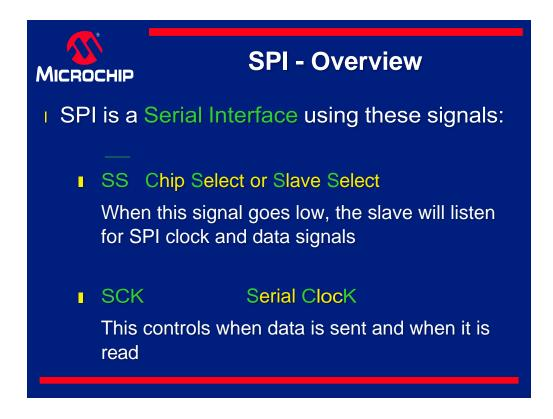
SPI is a Serial Interface and uses the following signals to serially exchange data with another device:
