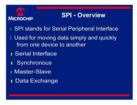
SPI stands for Serial Peripheral Interface.
