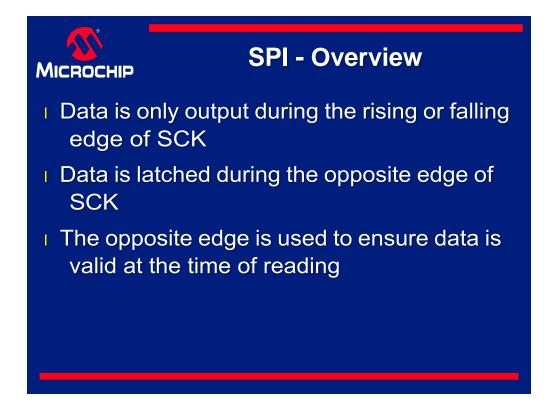
In SPI, data typically changes during the rising or falling edge of SCK. This is how the data is synchronized with the clock signal.
