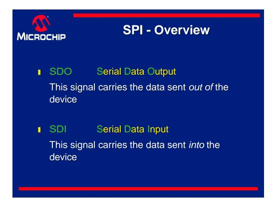
SDO - This is the Serial Data Output signal. SDO carries data out of a device.
