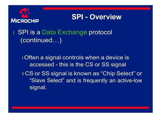
Often a slave select signal will control when a device is accessed. This signal must be used for when more than one slave exists in a system, but can be optional when only one slave exists in the circuit. As a general rule, it should be used.
