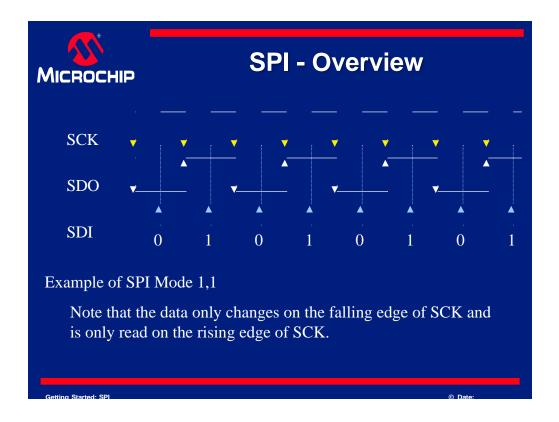
Here is an example of SPI communication. The arrows indicate whether the signal is experiencing a rising or falling edge at the time. SDI shows when the data is sampled.
