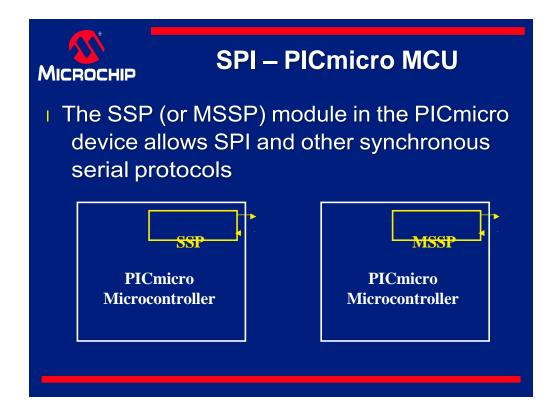
In the PICmicro device, a module is used for the SPI protocol. This module is named the SSP or MSSP module and allows SPI or  $I^2C$  to be implemented.
