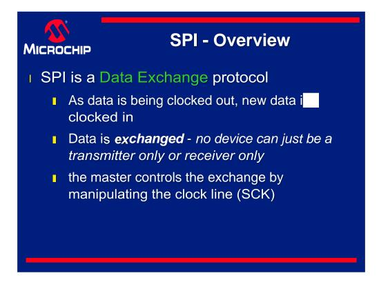
SPI is a Data Exchange protocol. As data is being clocked out, new data is also being clocked in.
