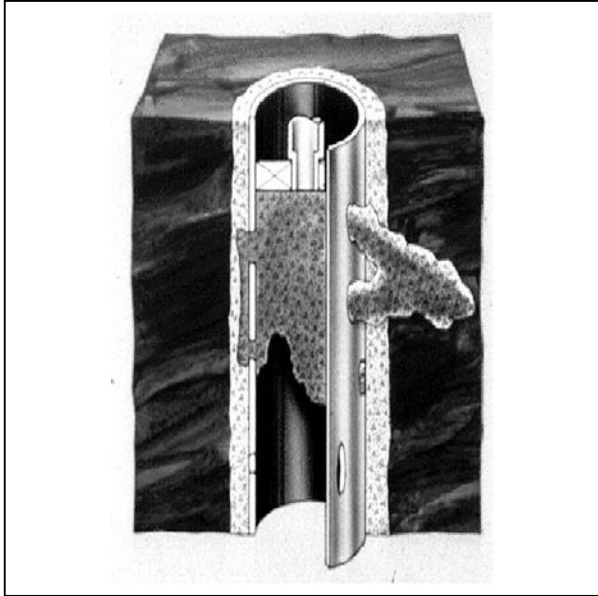
Figure 8.1 – Squeezing to repair casing.
