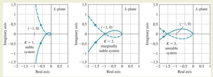
Angle of  $L(j\omega)$  is always -180° or less, and the locus of  $L(j\omega)$  is above
