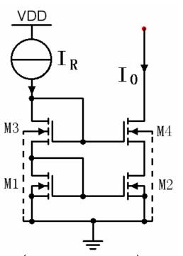
$$\frac{I_{O}}{I_{R}} = \frac{K_{2}W_{2}L_{1}(V_{GS2} - V_{T2})^{2}(1 + |\lambda_{2}V_{DS2}|)}{K_{1}W_{1}L_{2}(V_{GS1} - V_{T1})^{2}(1 + |\lambda_{1}V_{DS1}|)}$$
