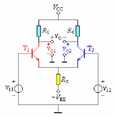
$$v_0 = (v_{C1} + \Delta v_{C1}) - (v_{C2} + \Delta v_{C2}) = 0$$
